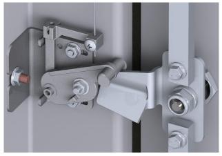
5. -INSTALL THE DEFEATER HOOK (ASSEMBLY 4) TO THE DOOR, AND ADJUST THE HEIGHT OF THE HOOK SO THAT IT WILL CLOSE OVER THE DEFEATER WITH THE DISCONNECT HANDLE IN THE OFF POSITION, ABOUT 1/8 INCH CLEARANCE.
