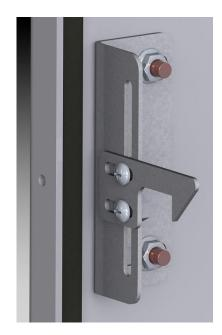
6. -NOW YOU CAN ADJUST THE MDV. WITH THE DISCONNECT OPERATING HANDLE STILL IN THE "OFF" POSITION SIMPLY PULL THE CABLE DRAWING DEFEATER STRIKE DOWN SO THAT THERE IS ABOUT A 3/8 INCH BETWEEN THE DEFEATER AND THE DEFEATER STRIKE AND TIGHTEN THE SCREW TO LOCK IN POSTION.
