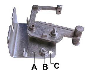
2. -INSERT (ASSEMBLY 1) OF THE "MDV" KIT BETWEEN THE ENCLOSURE FLANGE AND DISCONNECT MOUNTING PLATE AND TIGHTHEN THE FASTENERS, MAKING SURE THAT THE MDV LEVER MOVES FREELY UP AND DOWN.
